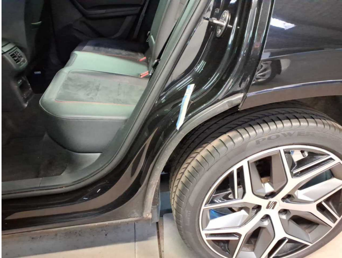
Damage 7: Side panel - rear left side: Side panel (Dichtung) - Broken / torn - Replace
