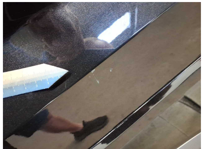
Damage 9: Door - rear left side: Door - Dent / paintcoat damage - Repair and paint
