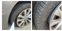
Damage Part: Tyre - RF Damage Type: Broken Repair Type: Replace Acceptable: No
