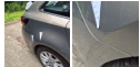
Damage Part: Fender - Rear Right Damage Type: Scratch(es) Repair Type: Spray Acceptable: No
