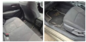
Damage Part: Interior Damage Type: Stains & dirt Repair Type: Cleaning Acceptable: No
