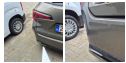
Damage Part: Bumper - Rear Damage Type: Small dent(s) Repair Type: PanelBeating & Spray Acceptable: No
