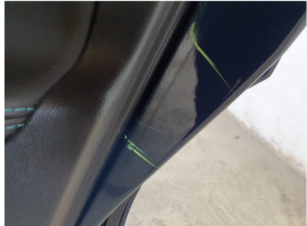
Damage #1: Door - rear right side: Door (Innen) - Dent / paintcoat damage - Smart repair
