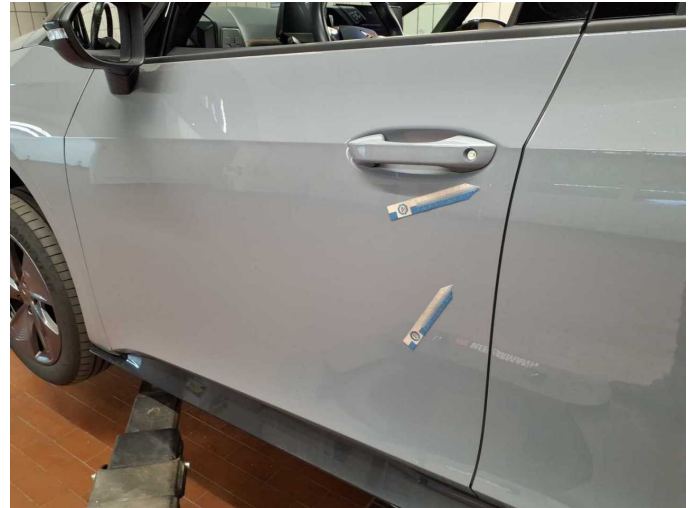
Damage 1: Door - front left side: Door - Dent / paintcoat damage - Repair and paint
