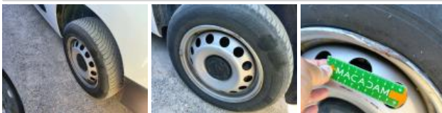
Steel rim FL, Not original part, Acceptable
