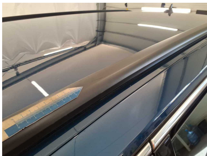
Damage 13: Roof: Roof (inkl. Railing) - Scratched - Paint
