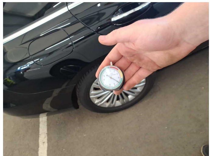
Damage 1: Wheel / tyres: Tyre - rear right side - Does not meet the leasing specifications - Replace
