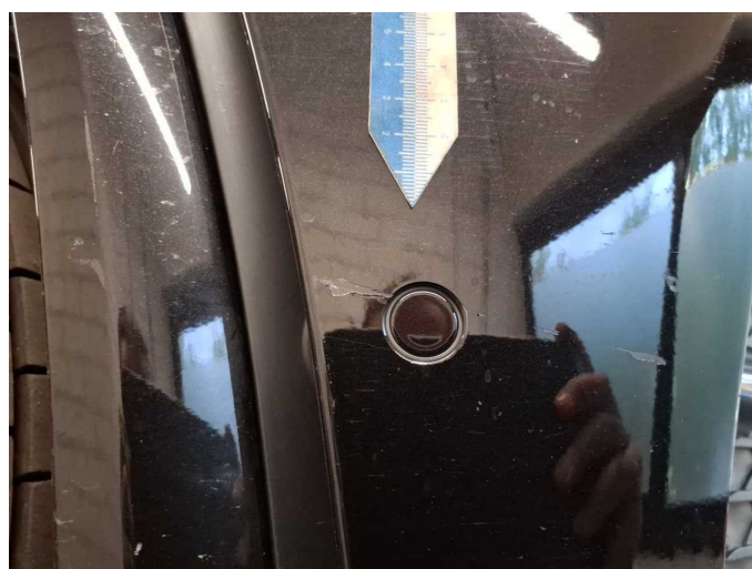
Damage 5: Front bumper: Bumper with Parktronic - Malposition - Set / adjust
