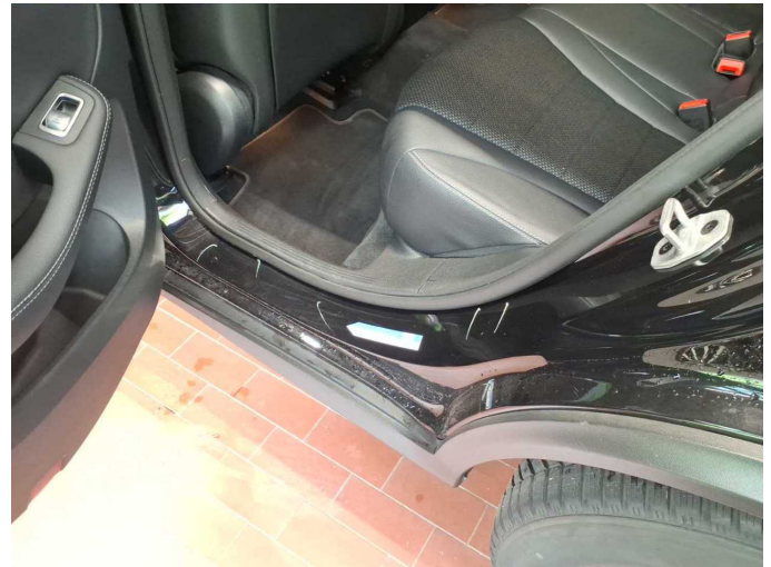
Damage 7: Side panel - rear left side: Sill - Dent / paintcoat damage - Smart repair
