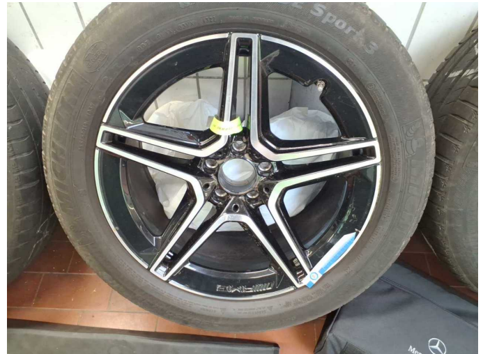
Damage 9: 2nd wheel set: 1 alloy rim (Hinten Rechts) - Scratch(es) - Loss in value
