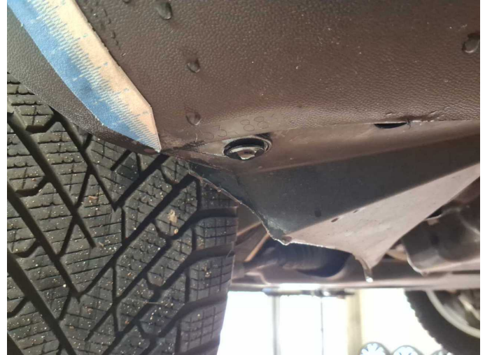
Damage 6: Mudguard - right side: Inner mudguard - Broken / torn - Replace
