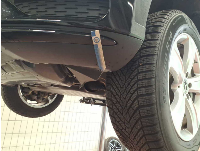
Damage 5: Mudguard - left side: Inner mudguard - Broken / torn - Replace
