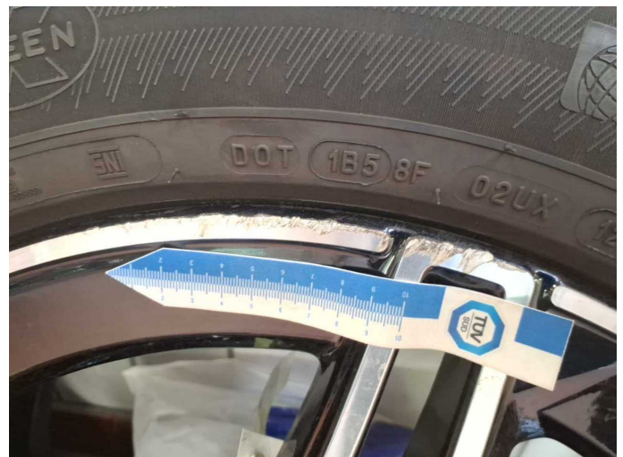
Damage 11: 2nd wheel set: 1 alloy rim (Vorne Rechts) - Scratched - Replace
