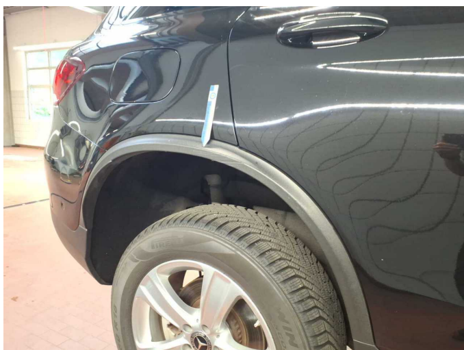
Damage 4: Side panel - rear right side: Wheel well extension - Scratch(es) - Replace
