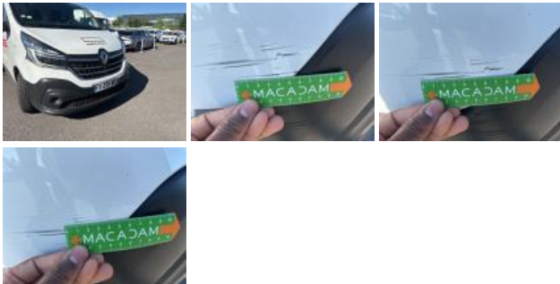
Bumper F, Scratch(es), Repair and paint (complete)
