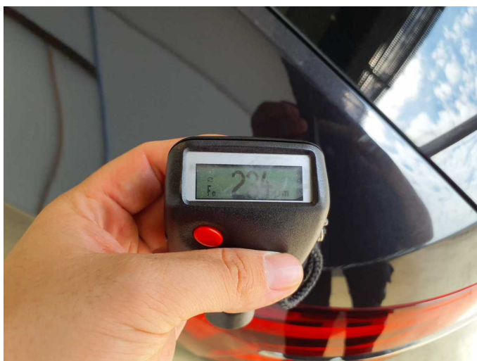
Repainting 1: Side panel - rear left side
