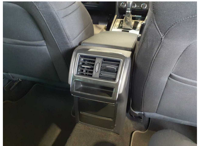
Damage 4: Instrument panel: Air nozzle - centre (Hinten) - Broken / torn - Replace
