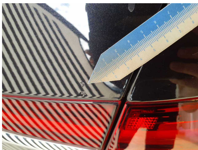
Damage 8: Boot lid / rear door: Boot lid - Corrosion - Repair and paint
