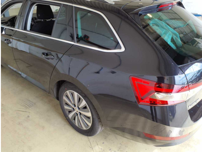
Damage 5: Side panel - rear left side: Side panel (Wellig) - Unprofessionally repaired - Repair and paint
