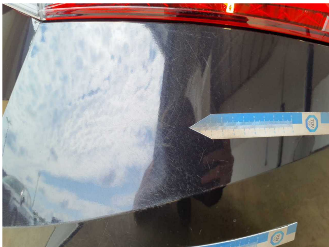
Damage 7: Rear bumper: Rear bumper - Scratch(es) - Paint
