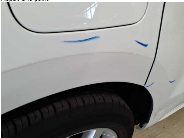
Damage #13: Side panel - rear right side: Side panel - Scratched - Repair and paint
