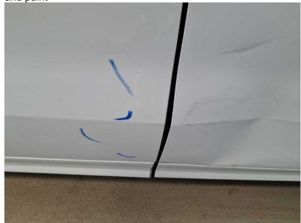
Damage #11: Sliding door, right: Sliding door with glass panel - Dent / paintcoat damage - Repair and paint
