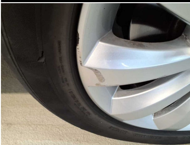
Damage #6: Wheel / tyres: Alloy rim - front right side - Scratched - Loss in value
