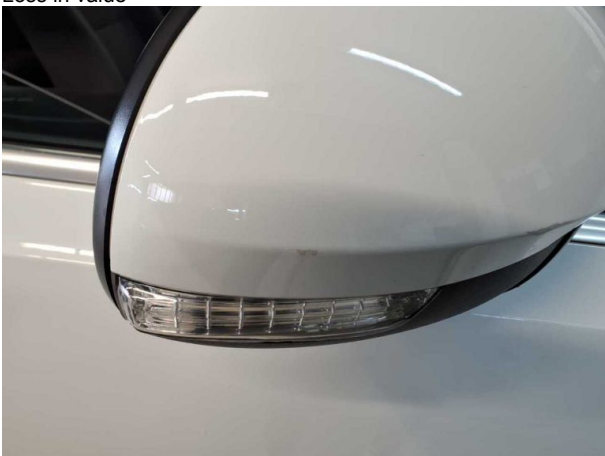
Damage #5: Wing mirror - right side: Cap - Scratched - Smart repair
