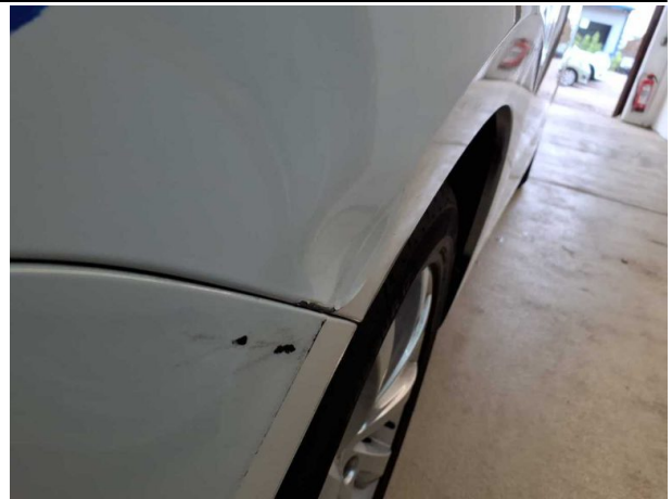
Damage #14: Mudguard - left side: Mudguard - left side - De... paintcoat damage - Replace
