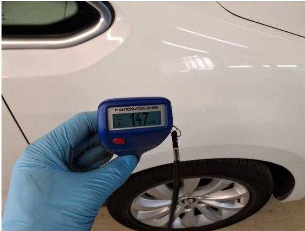
Repainting 1: Mudguard - right side, Door - front right side
