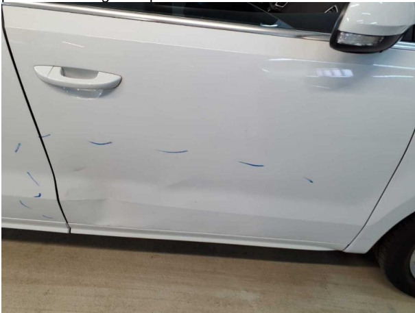
Damage #15: Door - front right side: Door - Deformed - Replace
