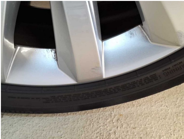
Damage #7: Wheel / tyres: Alloy rim - front left side - Scratched - Loss in value
