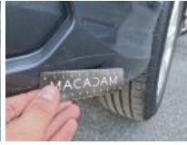
Bumper moulding R, Scratch(es), Paint
