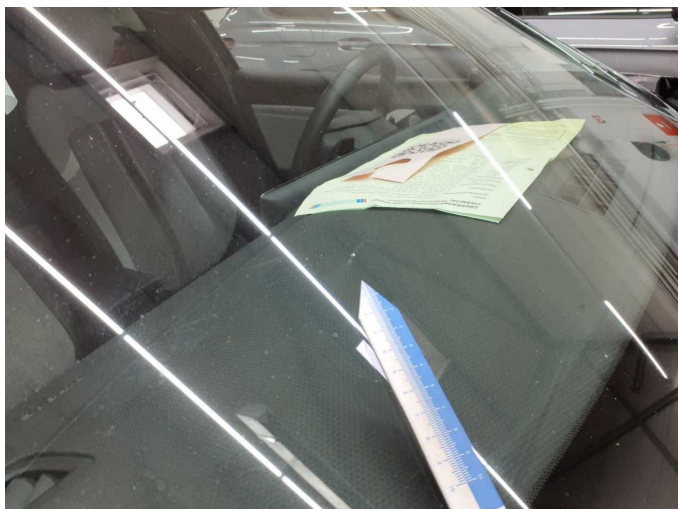
Damage 2: Vehicle glazing: Windscreen with lane departure assistant - Stone chips - Smart repair
