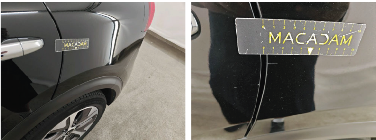
Wing RL Scratch(es) Repair and paint (complete) Left
