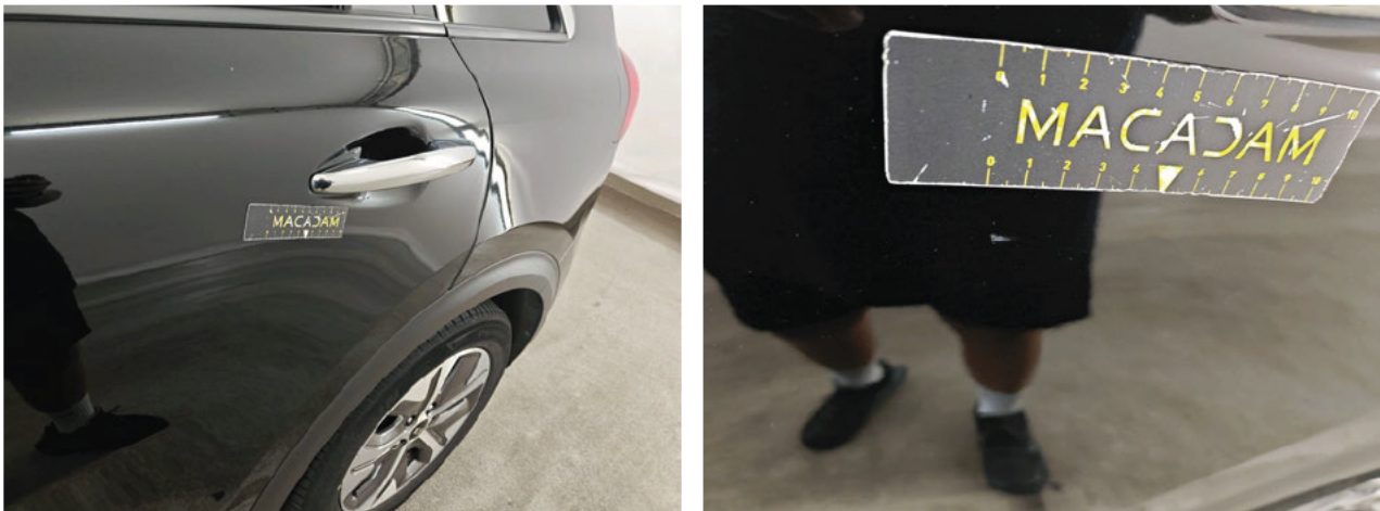
Door RL Scratch(es) Repair and paint (partial) Left
