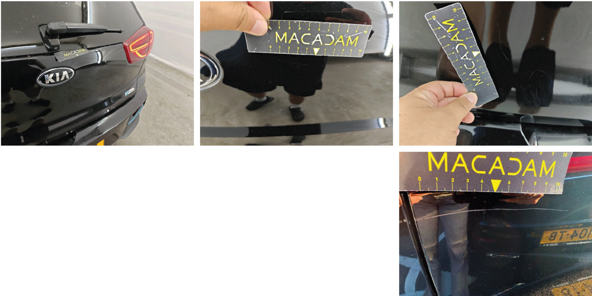
Wing RL Scratch(es) Repair and paint (complete) Left
