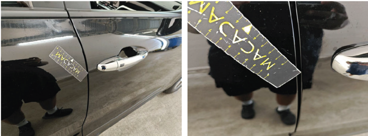
Door RR Scratch(es) Repair and paint (partial) Right
