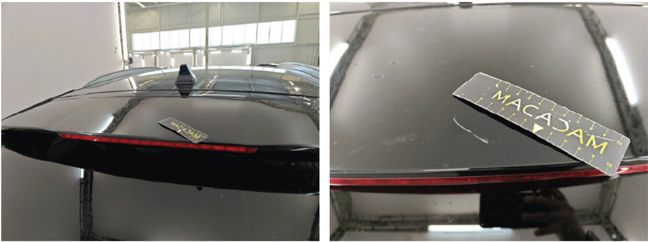
Rear spoiler Scratch(es) Repair and paint (complete) Rear
