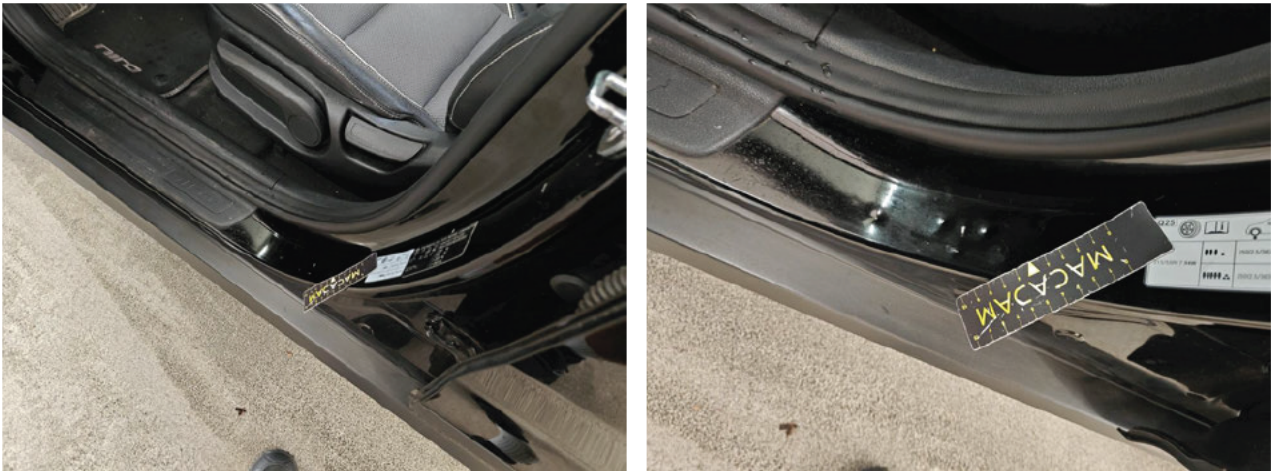
Door frame FL Dent(s) and scratch(es) Repair and paint (complete) Left
