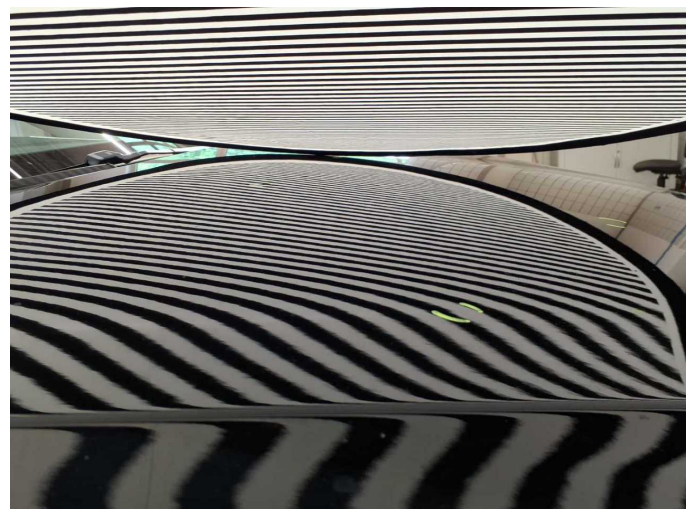
Damage 9: Bonnet: Bonnet - dent(s) - Smooth repair work
