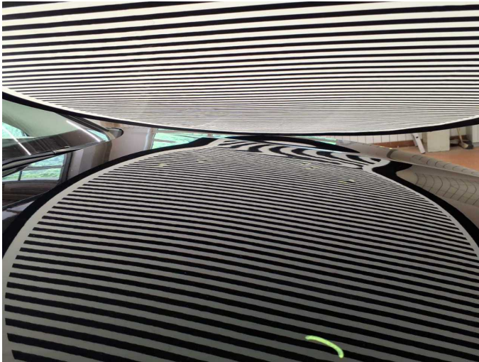
Damage 9: Bonnet: Bonnet - dent(s) - Smooth repair work
