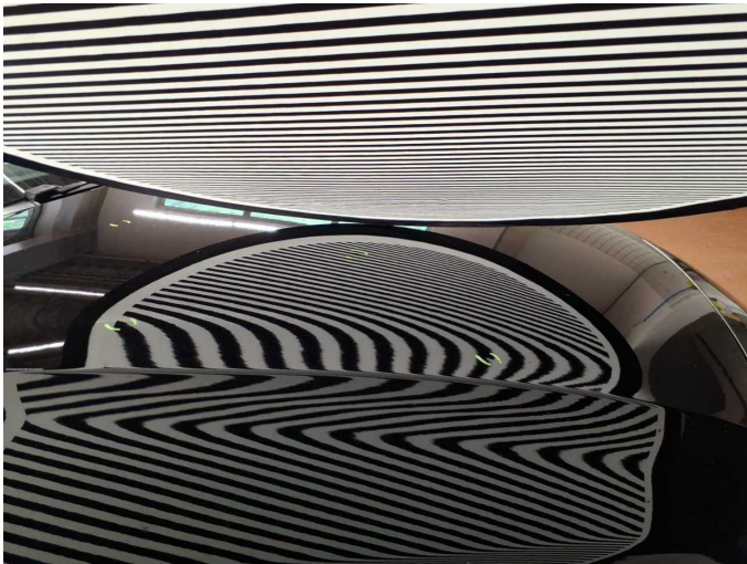
Damage 9: Bonnet: Bonnet - dent(s) - Smooth repair work
