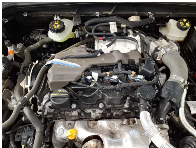
Missing part 1: Engine: Engine cover - Missing - Replace
