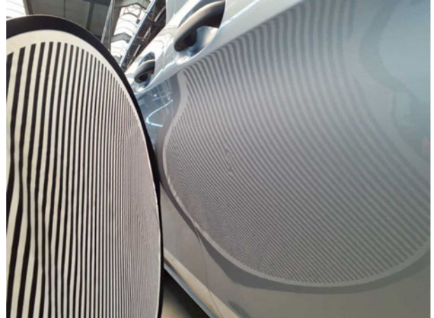
Beschädigung #1: Tür vorn rechts: Tür - Delle / Lackschaden - Smart Repair
