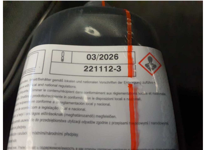
Damage 3: Equipment: Tirefit filler - Expired - Replace
