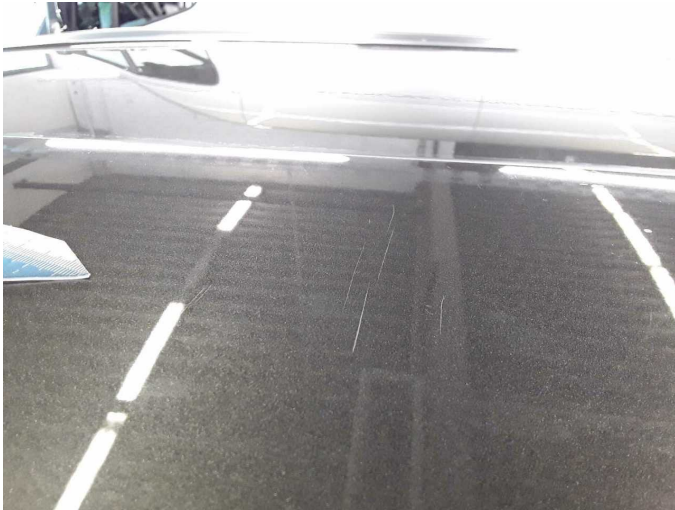
Damage 6: Roof: Roof - Scratch(es) - Paint
