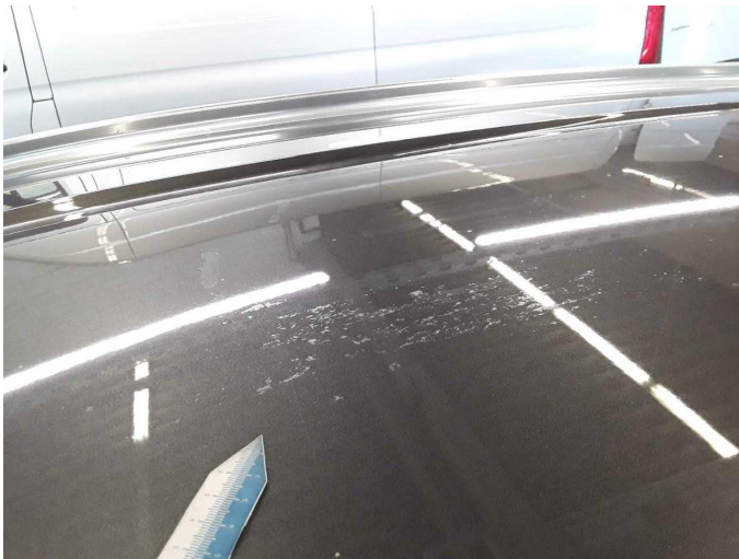
Damage 6: Roof: Roof - Scratch(es) - Paint
