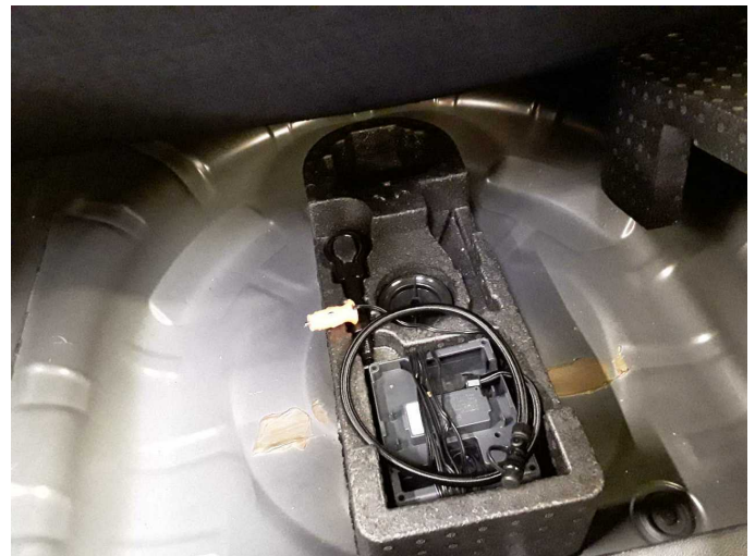
Missing part 1: Equipment: Tirefit filler - Missing - Replace
