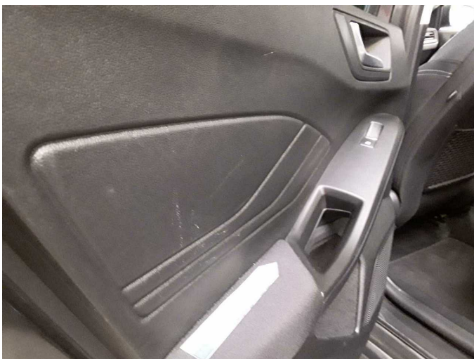
Wear and tear 1: Trim / covers: Door trim - rear left side - Scratch(es) - No deduction
