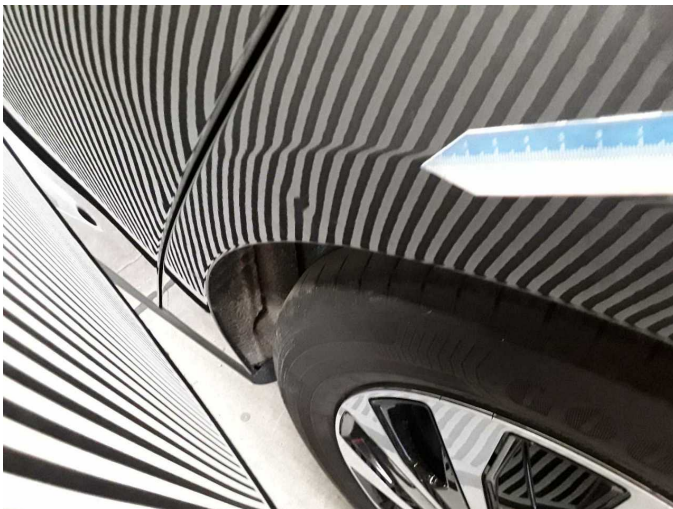
Damage 5: Side panel - rear left side: Side panel - Dent / paintcoat damage - Repair and paint
