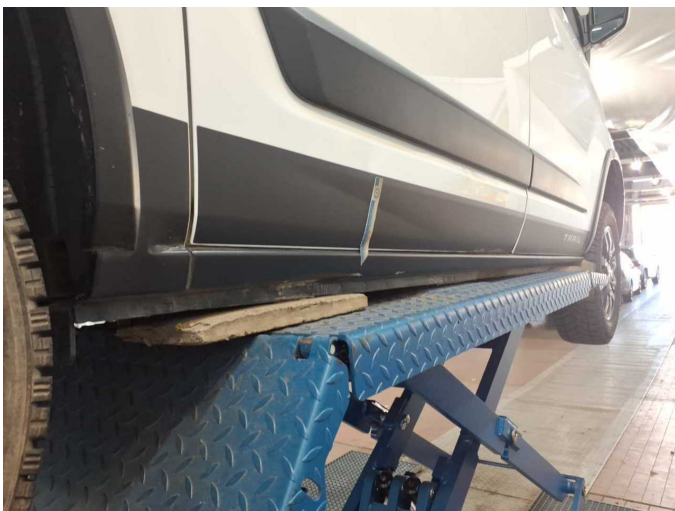
Damage 13: Sill - right side: Sill - Dent / paintcoat damage - Repair and paint
