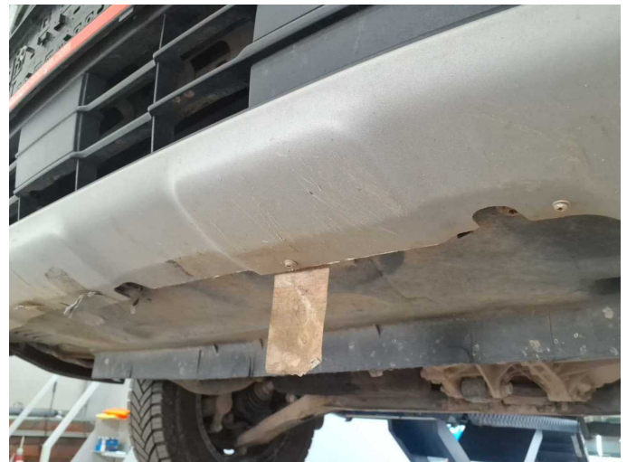
Damage 11: Front bumper: Spoiler (Mitte) - Deformed - Replace
