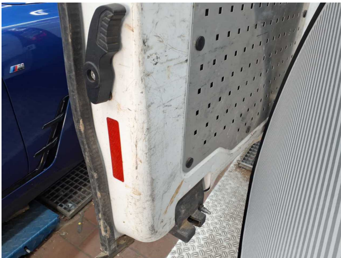
Damage 9: Boot lid / rear door: Rear door - right side (Und links) - Dent / paintcoat damage - Loss in value
