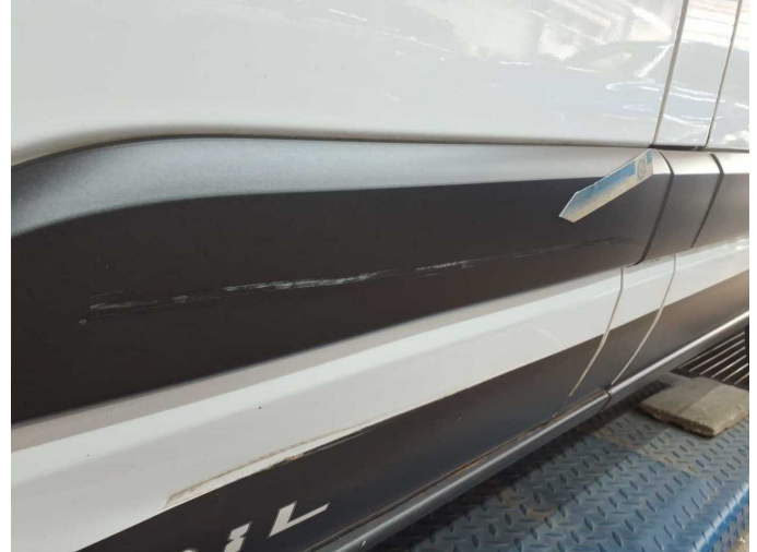
Damage 2: Door - front left side: Brightware - lower - Scratch(es) - Replace
