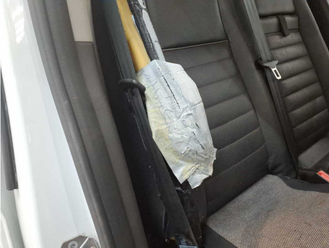
Damage 10: Seat - front: Backrest cover - 2 seater - right side - Broken / torn - Replace
