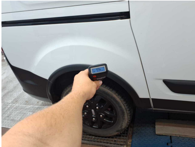
Repainting 1: Roof rail - right side, Mudguard - right side, Side panel - rear right side, Door - rear right side, Door - front right side
