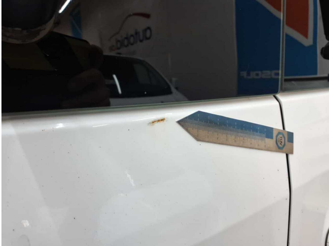
Damage 6: Boot lid / rear door: Rear door - left side (Außen) - Dent / paintcoat damage - Smart repair
