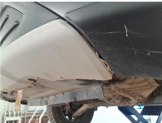
Damage 11: Front bumper: Spoiler (Mitte) - Deformed - Replace
