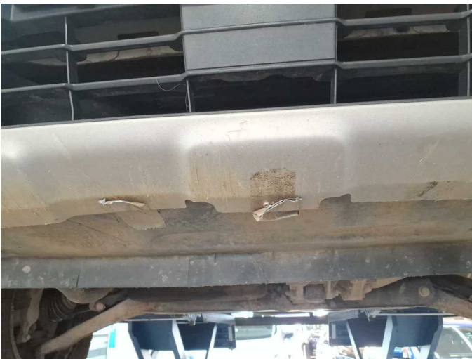
Damage 11: Front bumper: Spoiler (Mitte) - Deformed - Replace
