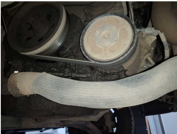
Damage 5: Engine: Engine - Leaking - Perform diagnosis
