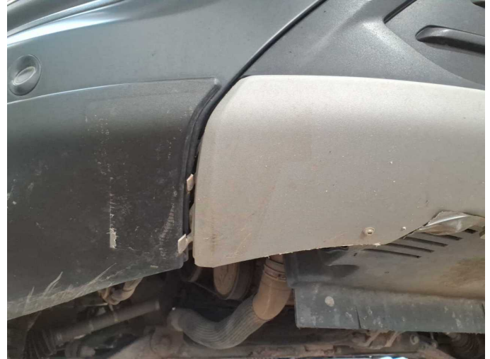
Damage 11: Front bumper: Spoiler (Mitte) - Deformed - Replace
