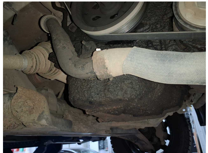
Damage 5: Engine: Engine - Leaking - Perform diagnosis
