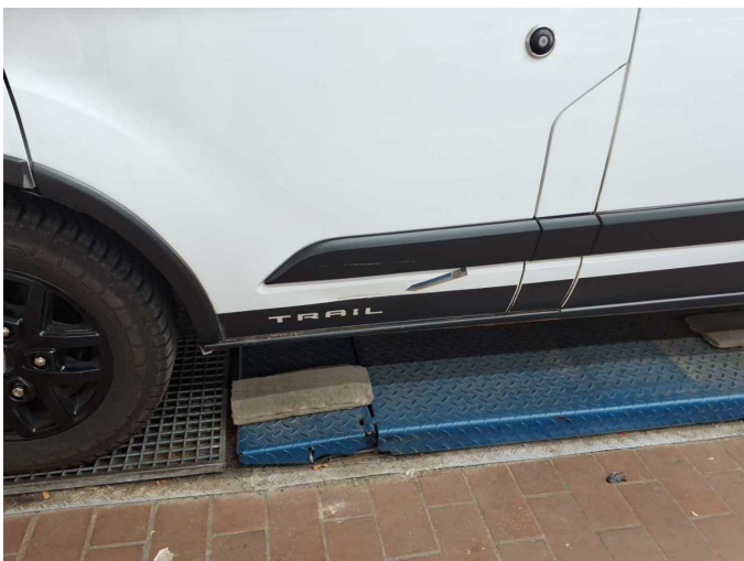
Damage 8: Door - front left side: Door - Dent / paintcoat damage - Smart repair
