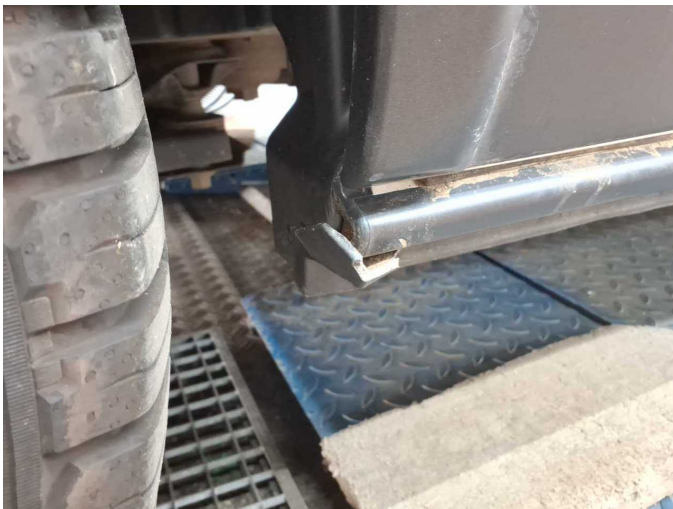
Damage 3: Mudguard - left side: Wheel arch (Spritzschutz) - Broken / torn - Replace
