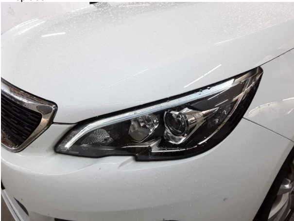
Damage #3: Headlight: Headlight - left side (Abblendlicht) - Non-operational - Replace
