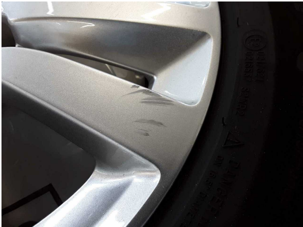
Damage #6: 2nd wheel set: 1 alloy rim - Scratched - Loss in value
