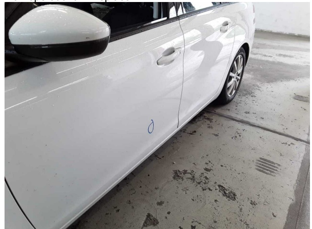
Damage #5: Door - front left side: Door - dent(s) - Smooth repair work
