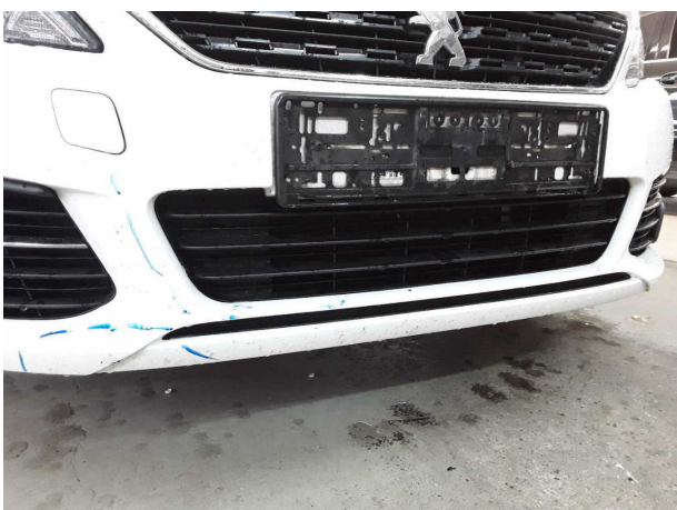
Damage #7: Front bumper: Grille - Loose - Diagnosed and repair if necessary
