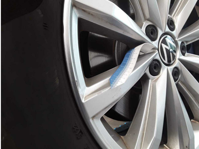
Damage 3: Wheel / tyres: Alloy rim - front right side - Scratch(es) - Loss in value
