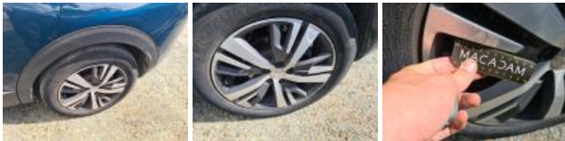
Tyre RR, Out of tolerance, Replace
