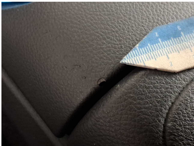
Damage 2: Interior: Interior - Broken / torn - Smart repair
