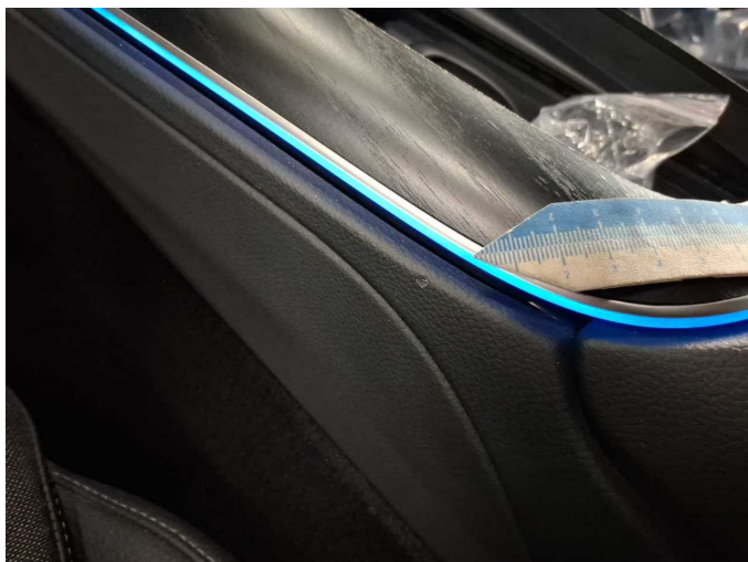
Damage 2: Interior: Interior - Broken / torn - Smart repair
