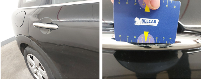
Door Rear Right / Door Handle / Replace-scratch
