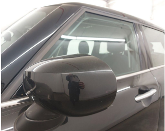
Side View Mirror Left // Painting-scratch
