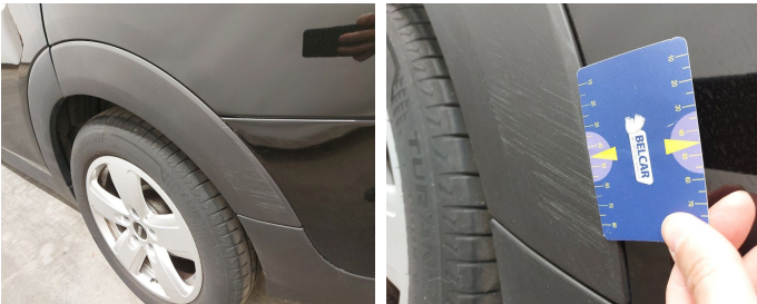
Wing Rear Left / Trim / Replace-scratch
