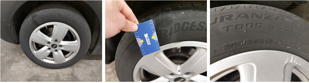
Tyre Rear Right // Replace-worn
