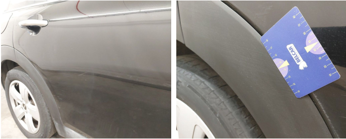
Door Rear Right / Trim / Replace-scratch
