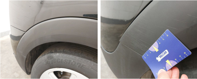
Wing Rear Right / Trim / Replace-scratch
