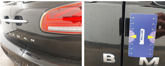
Rear Loading Door Right / Polish-scratch
