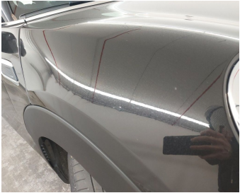
Wing Front right // Painting-scratch
