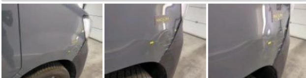
Side wall RR, Crack, Repair and paint (complete)
