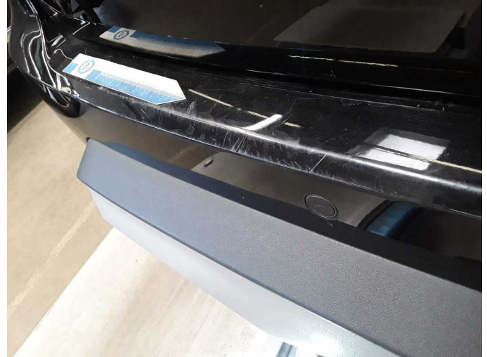
Damage 8: Rear bumper: Rear bumper - Scratch(es) - Paint
