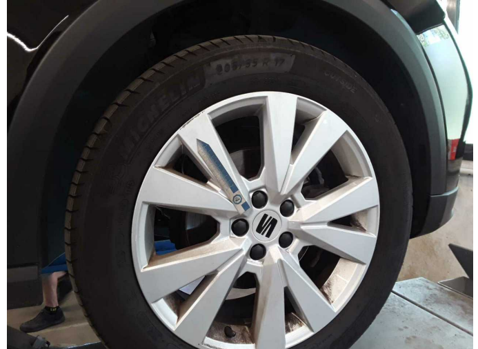
Damage 4: Wheel / tyres: Alloy rim - front right side - Scratch(es) - Smart repair
