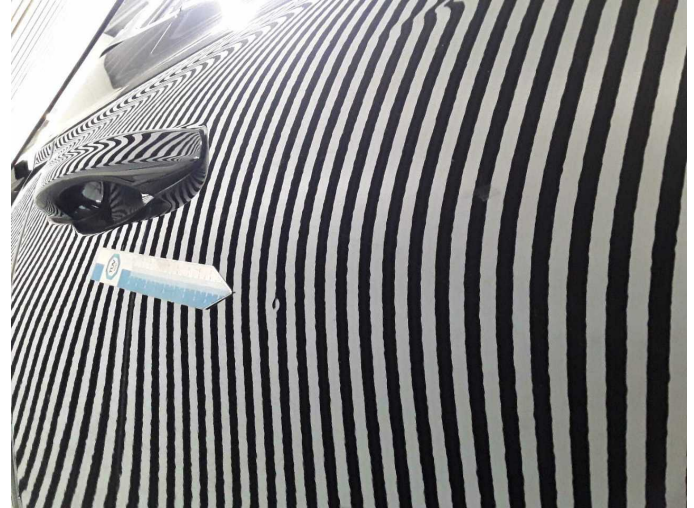
Wear and tear 2: Door - rear right side: Door - dent(s) - Smooth repair work
