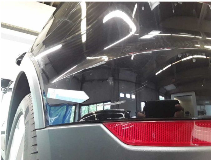
Damage 8: Rear bumper: Rear bumper - Scratch(es) - Paint
