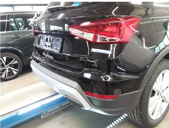
Damage 8: Rear bumper: Rear bumper - Scratch(es) - Paint
