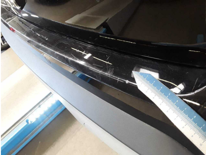
Damage 8: Rear bumper: Rear bumper - Scratch(es) - Paint
