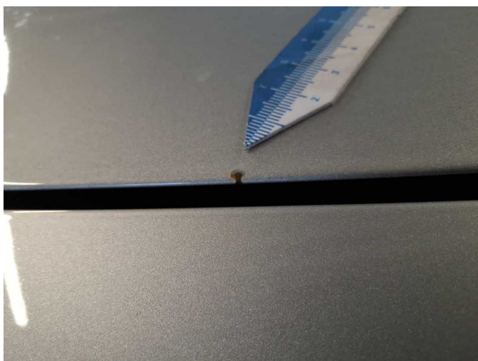
Damage 5: Bonnet: Bonnet (Korrosion) - Stone chips - Paint
