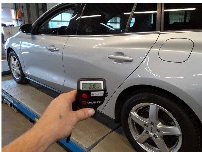
Repainting 3: Door - rear left side
