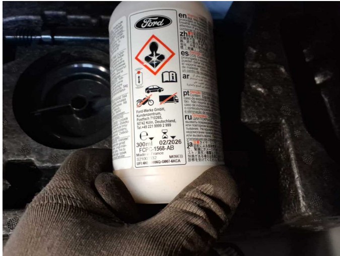
Damage 1: Equipment: Tirefit filler - Expired - Replace
