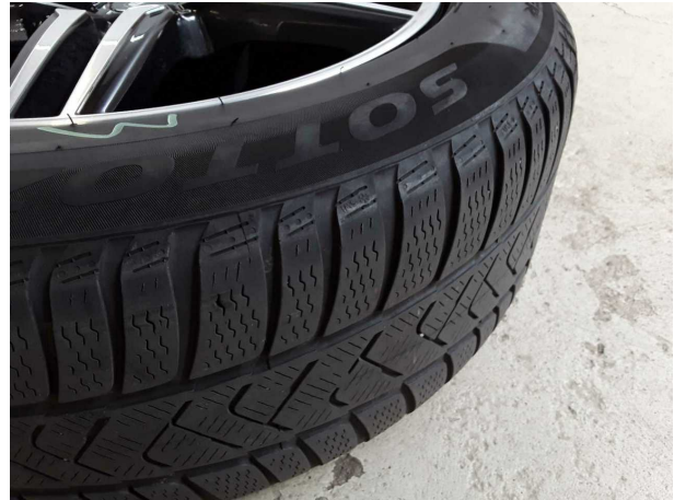
Damage #1: 2nd wheel set: 2 tyres - Worn - No deduction
