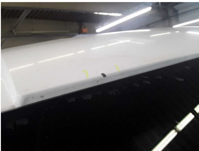
Damage 1: Roof: Roof - Stone chips - Smart repair
