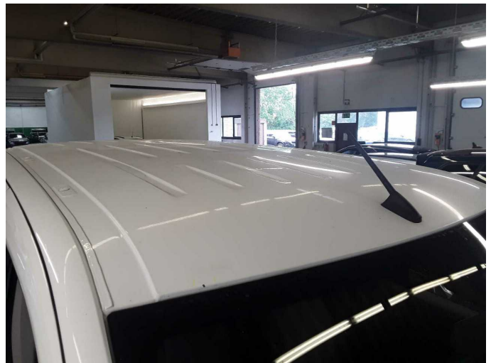
Damage 1: Roof: Roof - Stone chips - Smart repair
