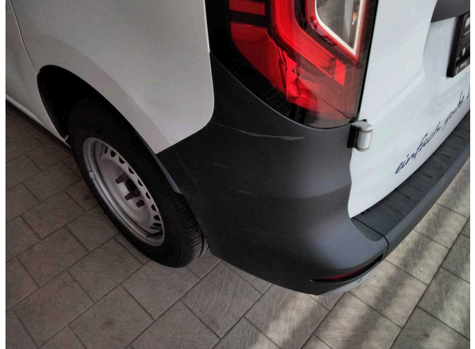
Damage 9: Rear bumper: Rear bumper - Scratch(es) - Loss in value
