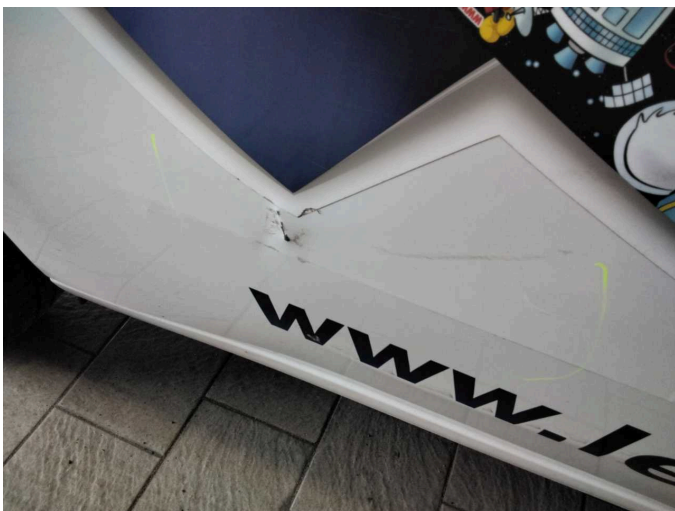
Damage 17: Sliding door, right: Sliding door with glass panel - Dent / paintcoat damage - Repair and paint
