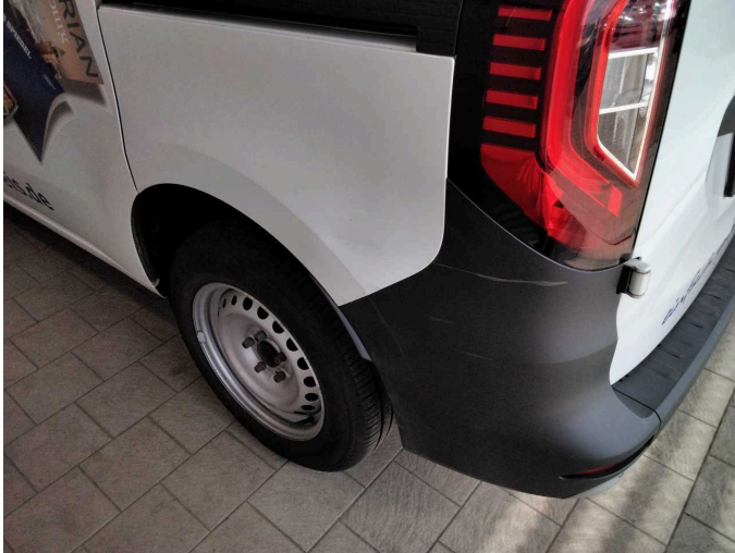
Damage 16: Side panel - rear left side: Side panel - Dent / paintcoat damage - Repair and paint
