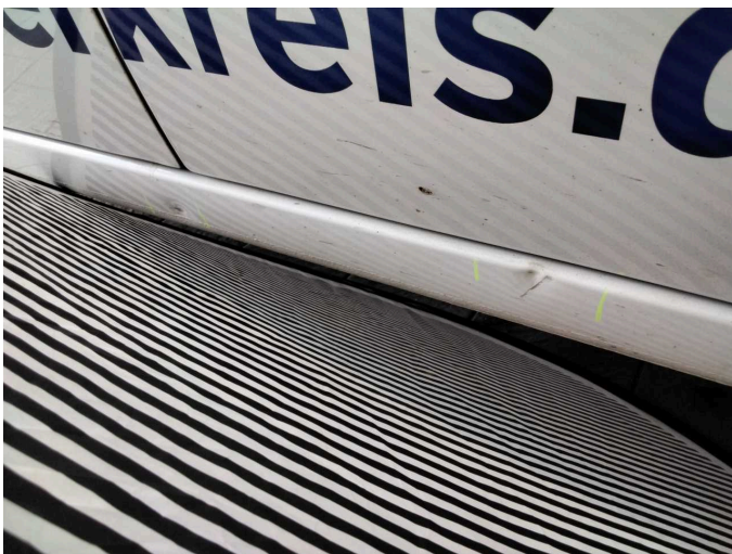
Damage 1: Sill - right side: Sill - dent(s) - Smooth repair work
