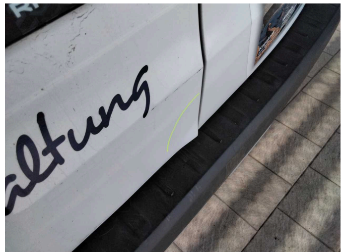
Damage 15: Boot lid / rear door: Rear door - left side - Deformed - Repair and paint
