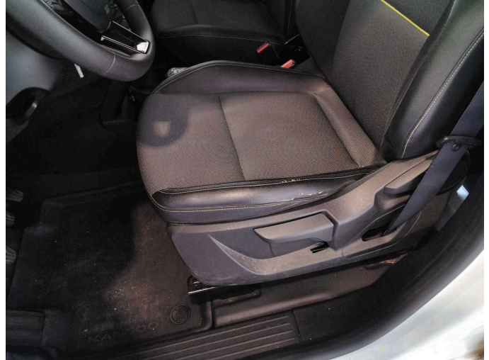
Damage 3: Seat - front: Seat cover - left side - Broken / torn - Smart repair
