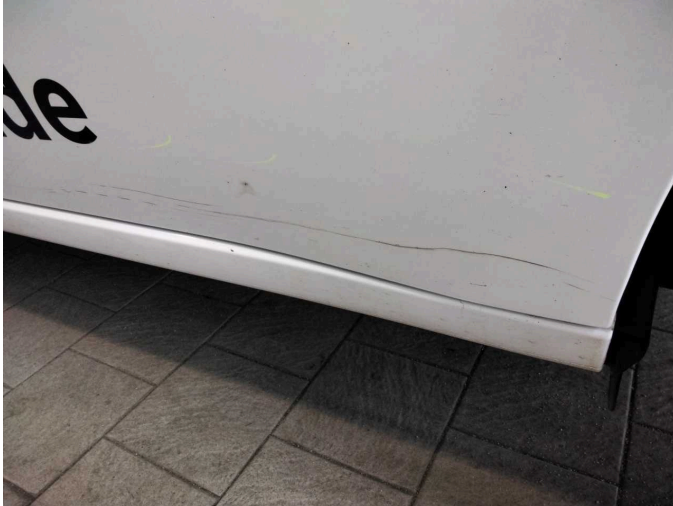
Damage 11: Sliding door - left side: Sliding door with glass panel (Unterhalb) - Scratch(es) - Smart repair
