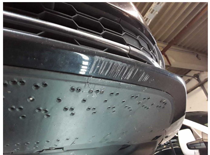
Damage 9: Front bumper: Front bumper - Scratched - Paint
