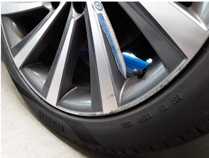
Damage 3: Wheel / tyres: Alloy rim - rear left side - Scratch(es) - Loss in value
