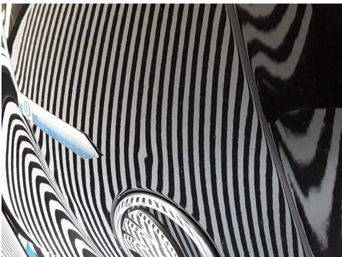
Damage 8: Bonnet: Bonnet - Dent / paintcoat damage - Paint
