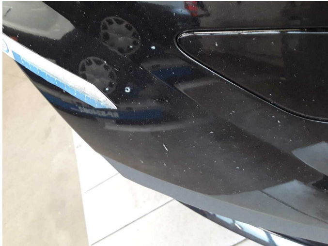
Damage 9: Front bumper: Front bumper - Scratched - Paint
