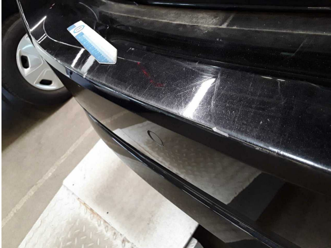
Damage 7: Rear bumper: Rear bumper - Scratch(es) - Paint
