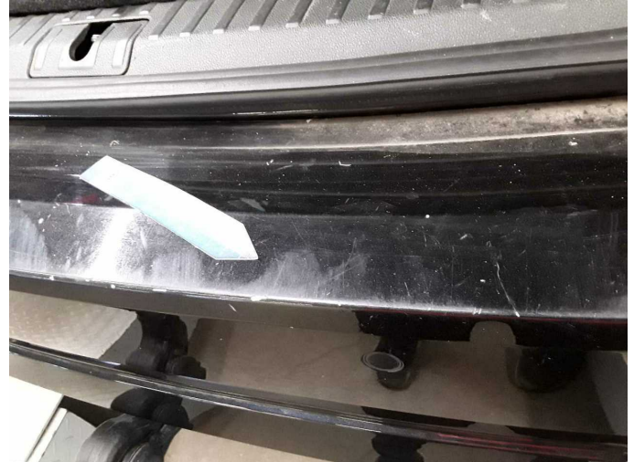
Damage 7: Rear bumper: Rear bumper - Scratch(es) - Paint
