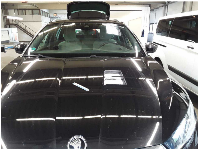
Damage 8: Bonnet: Bonnet - Dent / paintcoat damage - Paint
