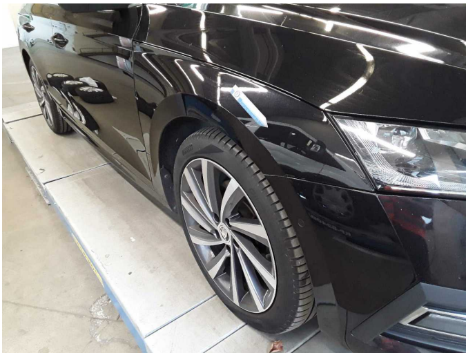
Damage 6: Mudguard - right side: Mudguard - right side - Dent / paintcoat damage - Paint
