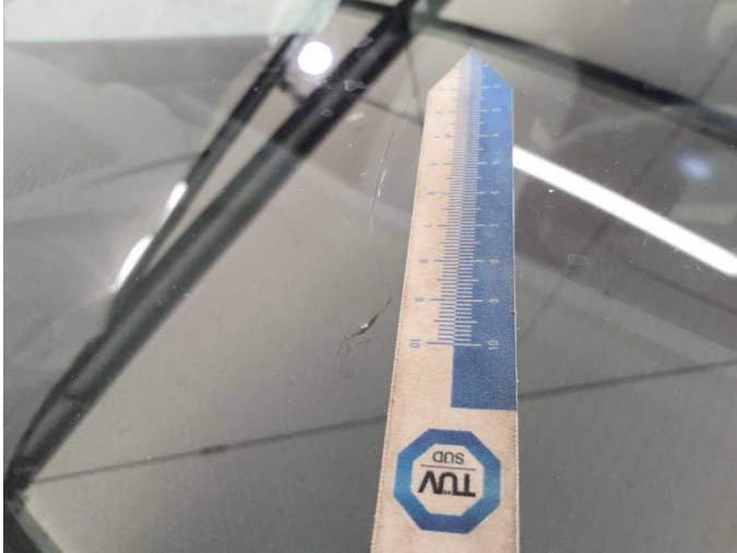
Damage 4: Vehicle glazing: Windscreen - Broken / torn - Replace
