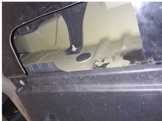
Damage 6: Rear of vehicle: Trailer hitch (Träger, Dose & Kugelkopf) - Missing - Replace
