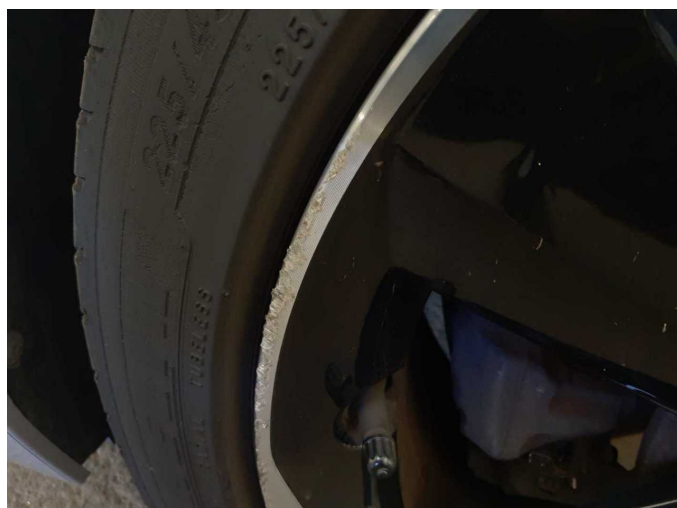
Damage 3: Wheel / tyres: Alloy rim - front left side - Scratched - Replace
