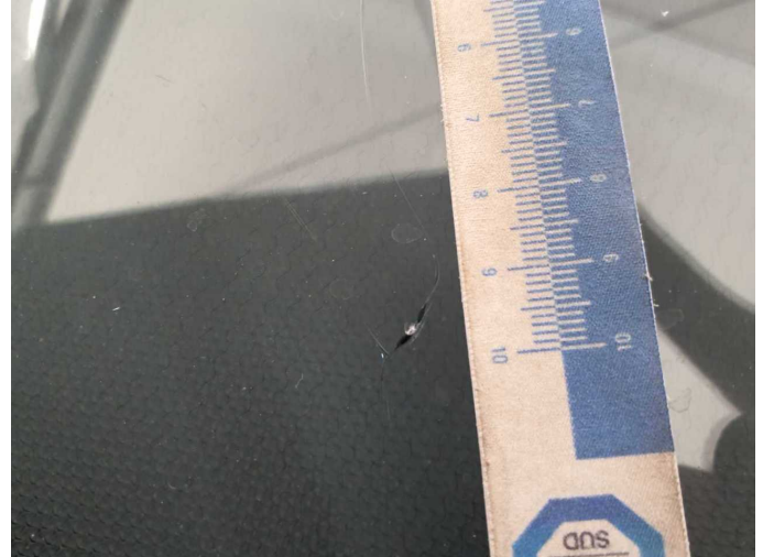
Damage 4: Vehicle glazing: Windscreen - Broken / torn - Replace
