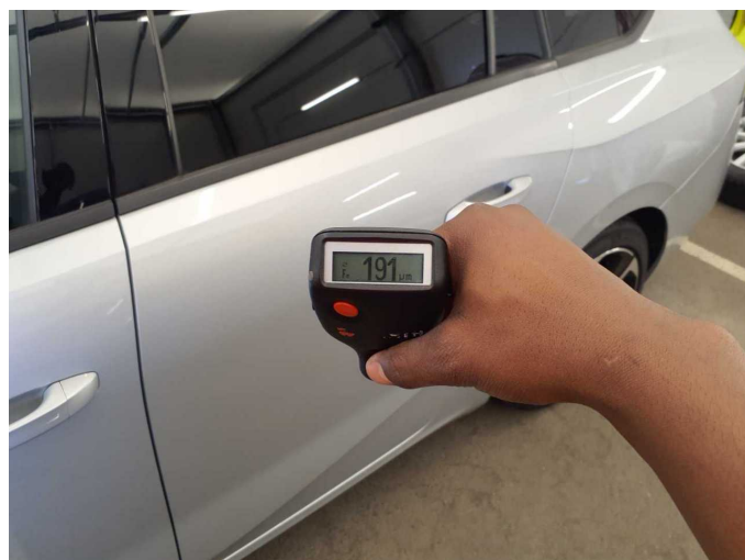
Repainting 1: Door - rear left side
