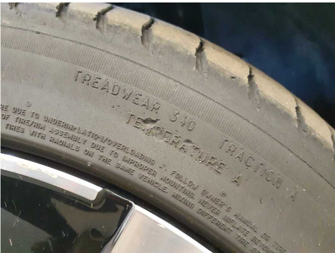
Damage 1: Wheel / tyres: Tyre - front left side - Broken / torn - Replace
