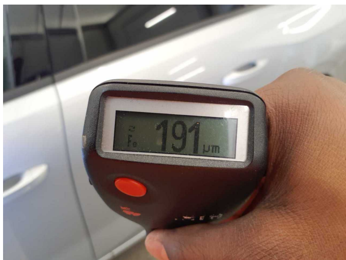
Repainting 1: Door - rear left side
