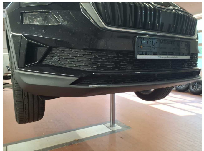
Damage 3: Front bumper: Spoiler - Scratched - Replace
