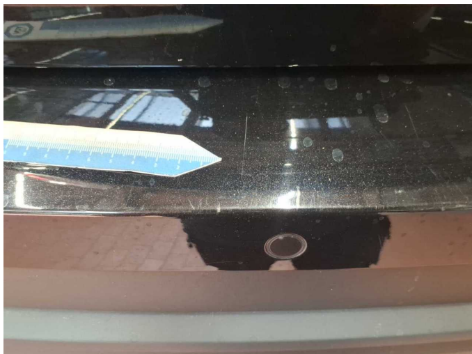
Damage 4: Rear bumper: Rear bumper - Scratch(es) - Paint
