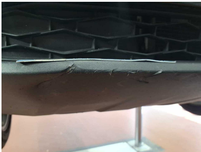
Damage 3: Front bumper: Spoiler - Scratched - Replace
