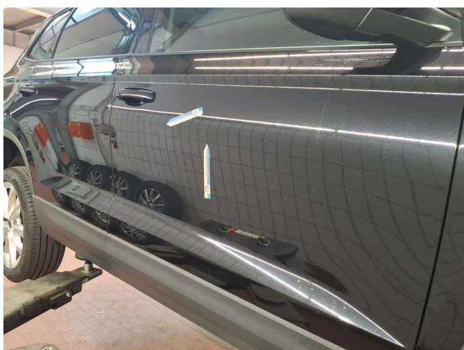
Wear and tear 2: Door - front right side: Door - Dent / paintcoat damage - No deduction
