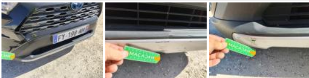
Bumper moulding F, Deformed / Strained, Replace
