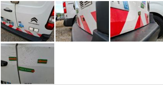
Bumper corner RR, Deformed / Strained, Replace
