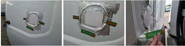
Side repeater R, Broken, Replace
