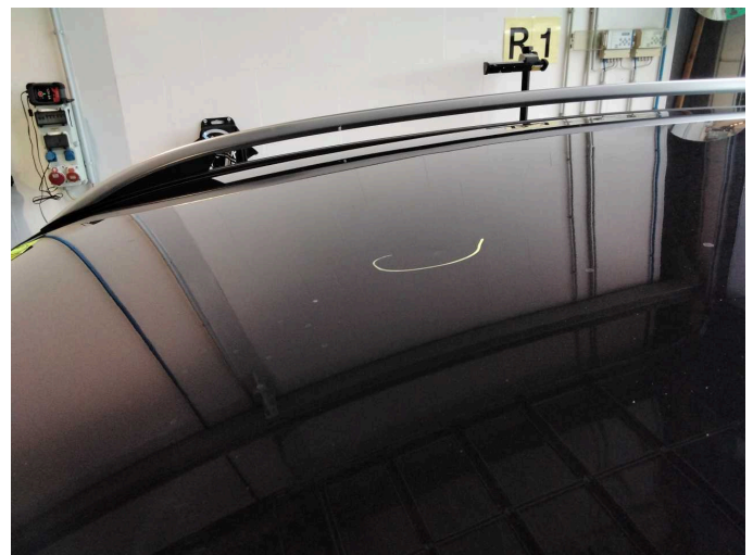
Damage 2: Roof: Roof - dent(s) - Smooth repair work
