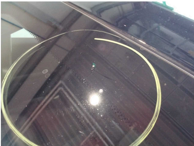
Damage 6: Vehicle glazing: Windscreen - Stone chips - Replace
