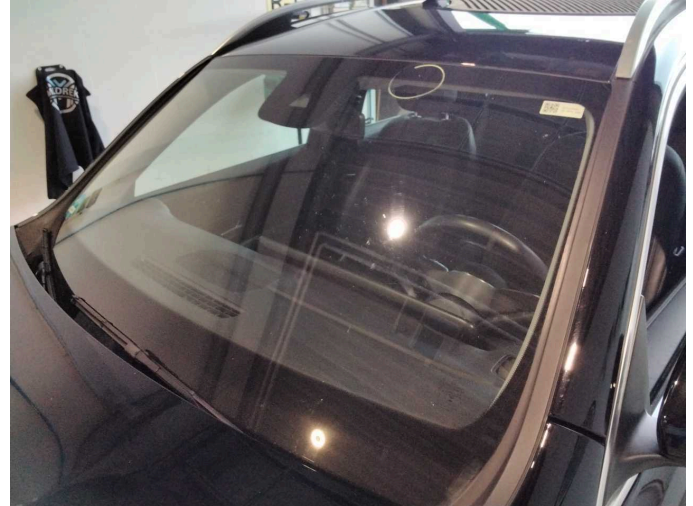
Damage 6: Vehicle glazing: Windscreen - Stone chips - Replace
