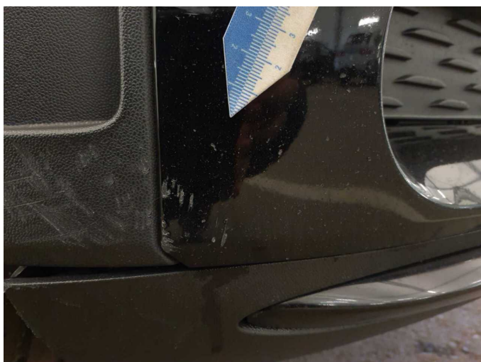
Damage 7: Front bumper: Front bumper - Scratch(es) - Paint
