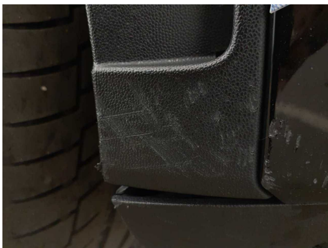
Damage 2: Front bumper: Bumper - front right side (Zierleiste) - Scratched - Replace
