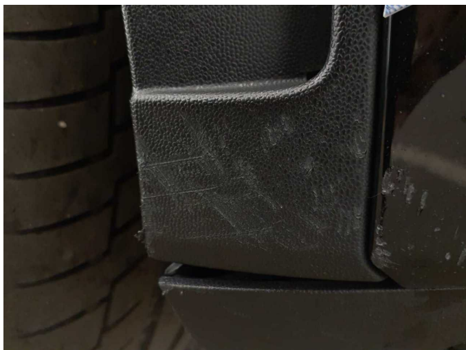
Damage 6: Mudguard - right side: Wheel arch - Scratched - Replace
