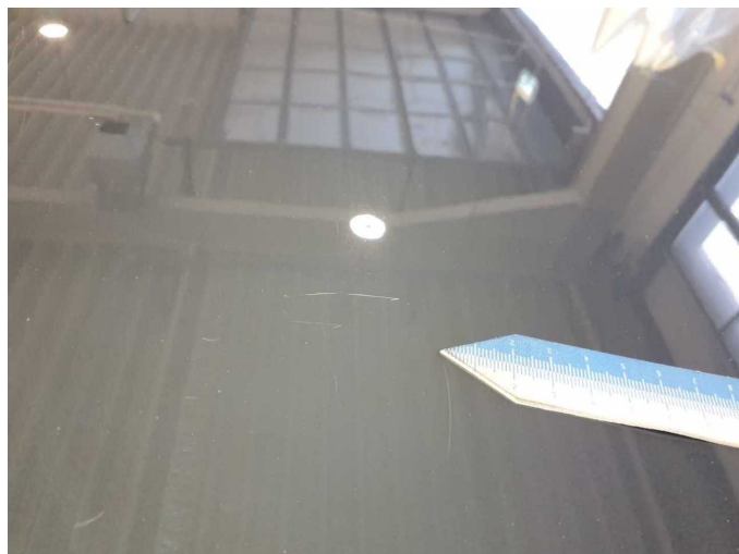
Damage 14: Roof: Roof - Scratch(es) - Paint
