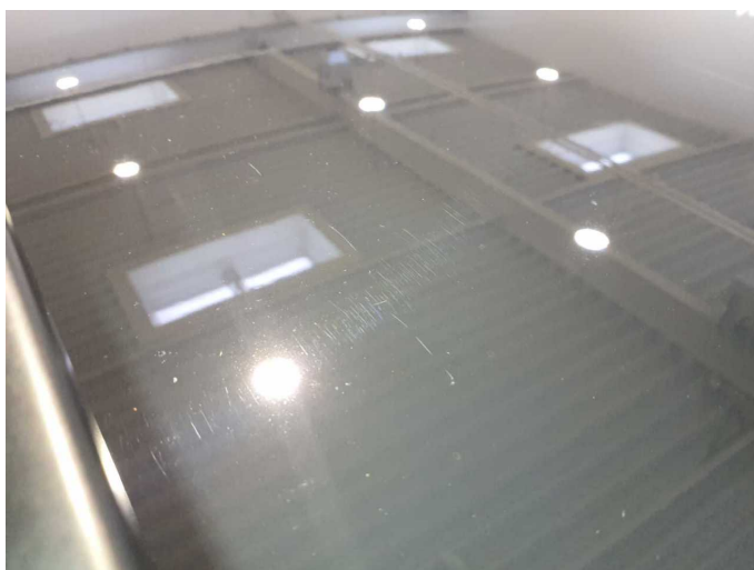
Damage 14: Roof: Roof - Scratch(es) - Paint
