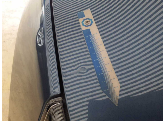
Damage 4: Bonnet: Bonnet - dent(s) - Smooth repair work
