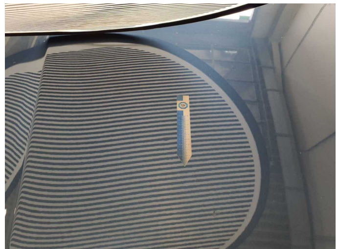
Damage 4: Bonnet: Bonnet - dent(s) - Smooth repair work
