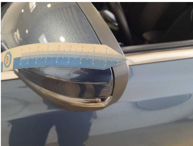
Damage 5: Wing mirror - left side: Cap - Scratch(es) - Smart repair
