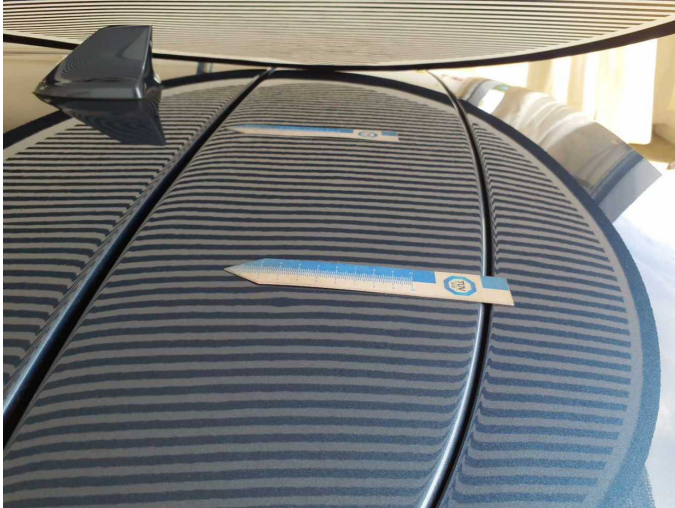
Damage 8: Boot lid / rear door: Rear spoiler - dent(s) - Repair and paint
