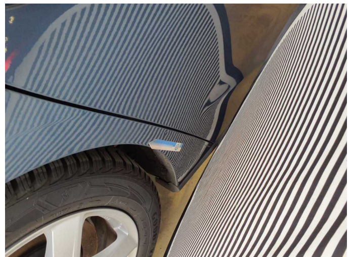
Wear and tear 7: Side panel - rear right side: Side panel - dent(s) - No deduction
