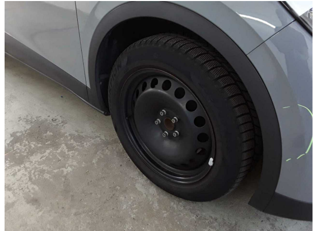
Damage #2: Wheel / tyres: Wheel cover - front right side (Original fehlt) - Replace
