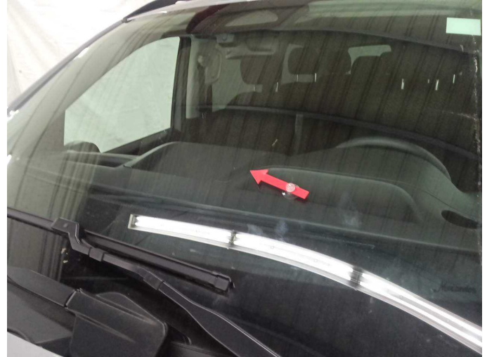
Wear and tear 1: Vehicle glazing: Windscreen - Stone chips - No deduction
