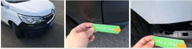
Grille, Broken, Replace
