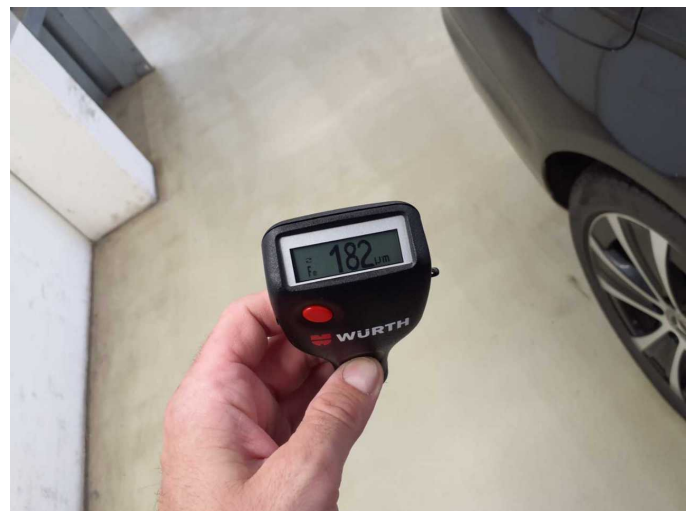
Roof rail - right side: 182 µm
