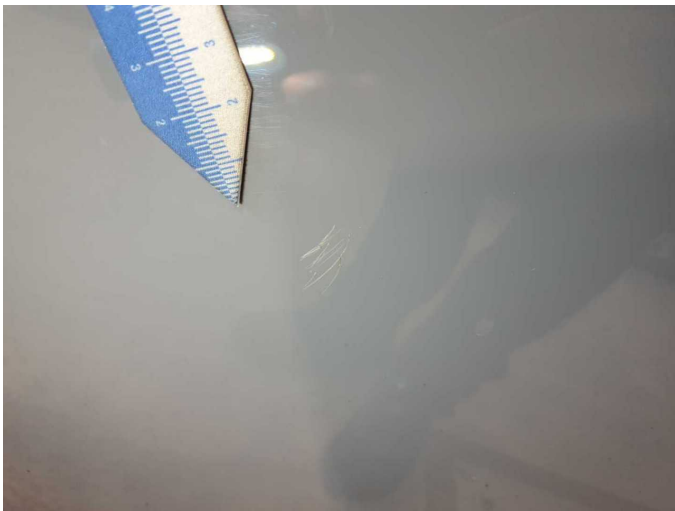
Damage 8: Door - front right side: Door - Scratch(es) - Paint
