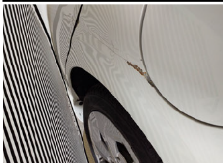
Kotflügel / Hinten Links / Delle
