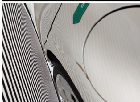
Kotflügel / Hinten Links / Delle
