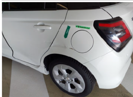
Kotflügel / Hinten Links / Delle
