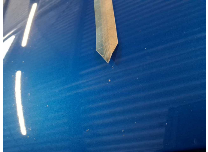
Damage 5: Bonnet: Bonnet - Dent / paintcoat damage - Paint
