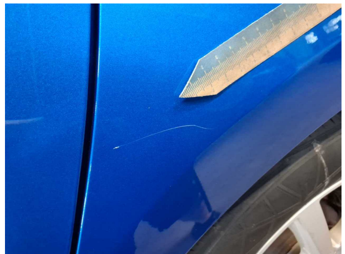
Damage 3: Side panel - rear left side: Side panel - Scratch(es) - Smart repair
