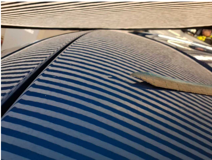
Damage 5: Bonnet: Bonnet - Dent / paintcoat damage - Paint
