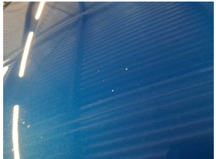
Damage 5: Bonnet: Bonnet - Dent / paintcoat damage - Paint
