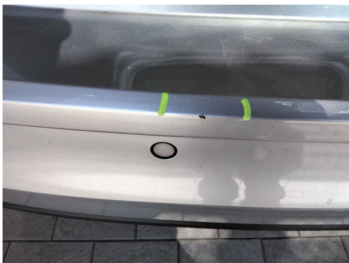
Damage 6: Rear bumper: Rear bumper - Scratch(es) - Paint
