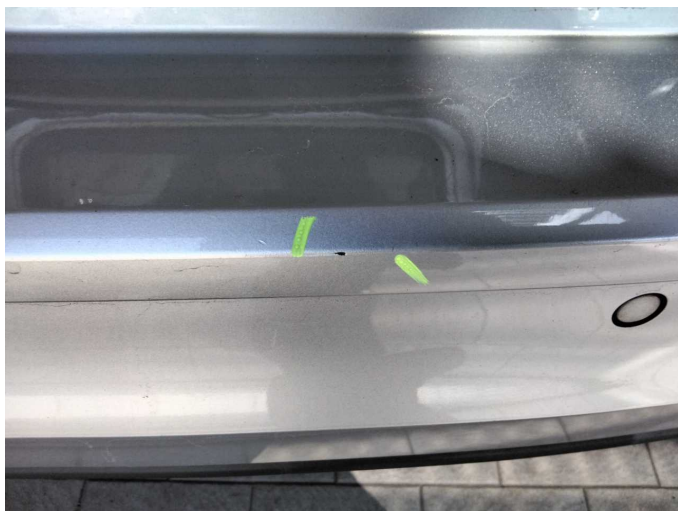
Damage 6: Rear bumper: Rear bumper - Scratch(es) - Paint
