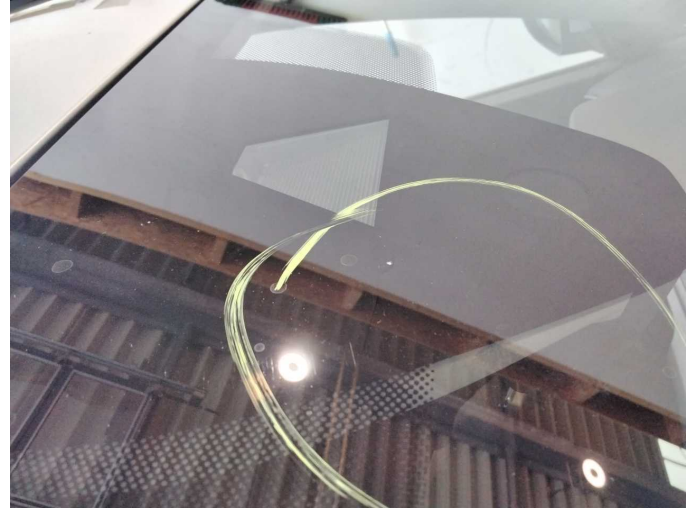
Damage 7: Vehicle glazing: Windscreen - Stone chips - Replace
