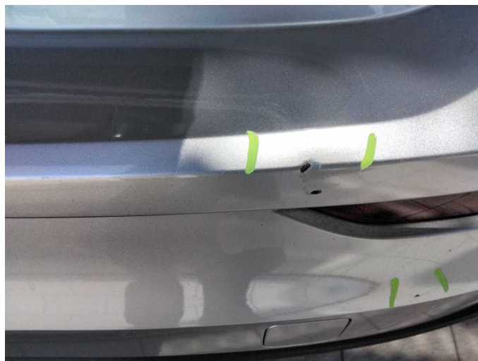
Damage 6: Rear bumper: Rear bumper - Scratch(es) - Paint
