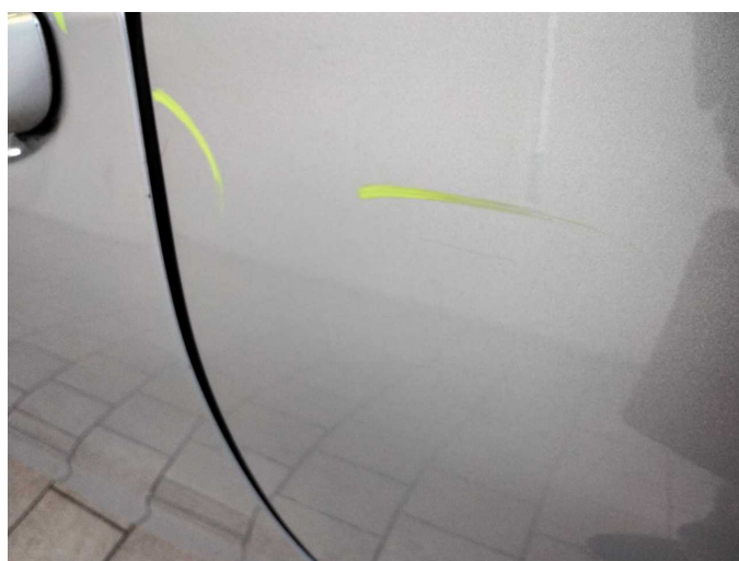
Damage 4: Door - rear left side: Door - Scratch(es) - Smart repair
