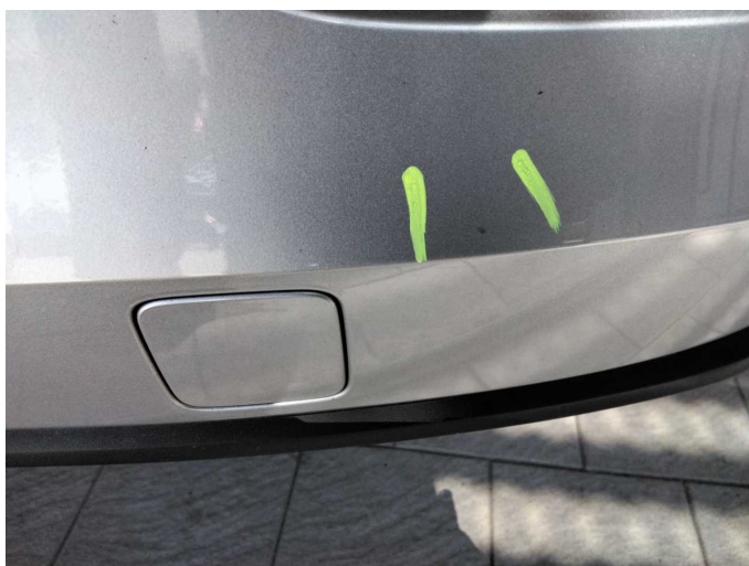
Damage 6: Rear bumper: Rear bumper - Scratch(es) - Paint
