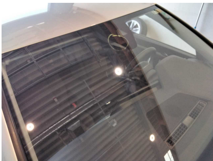
Damage 7: Vehicle glazing: Windscreen - Stone chips - Replace
