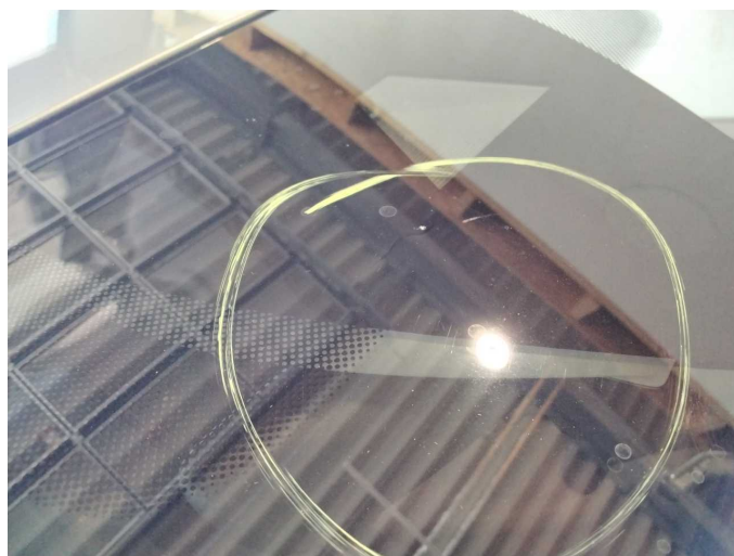
Damage 7: Vehicle glazing: Windscreen - Stone chips - Replace
