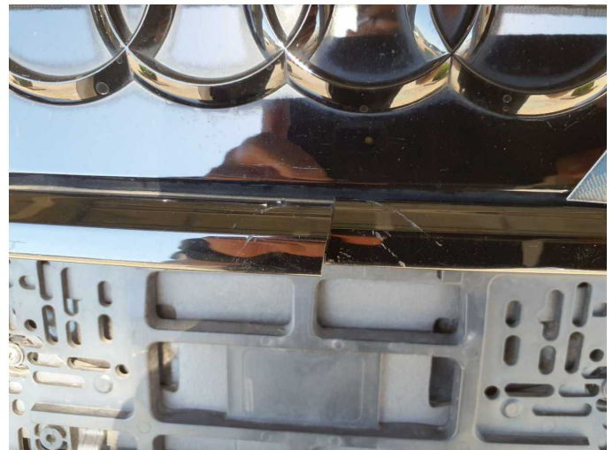
Damage 6: Trim / covers: Trim / covers (Zierleiste) - Broken / torn - Replace
