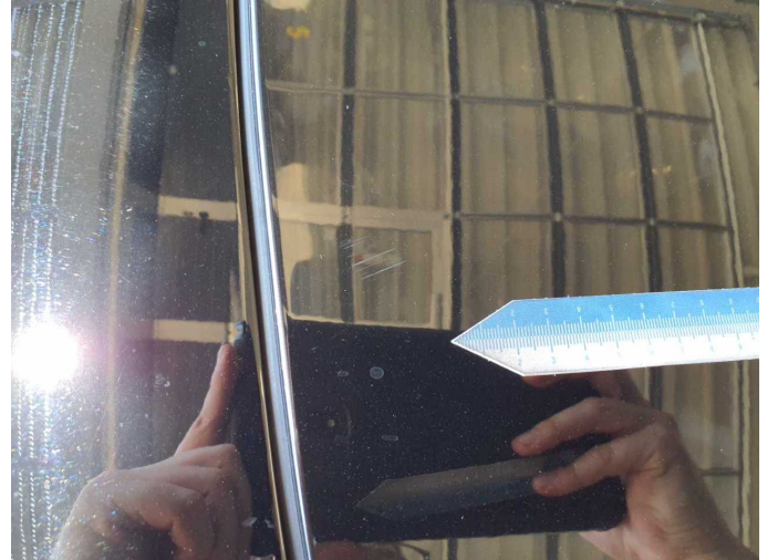
Damage 12: Roof: Roof - Scratch(es) - Paint
