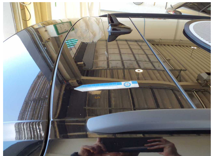
Damage 12: Roof: Roof - Scratch(es) - Paint
