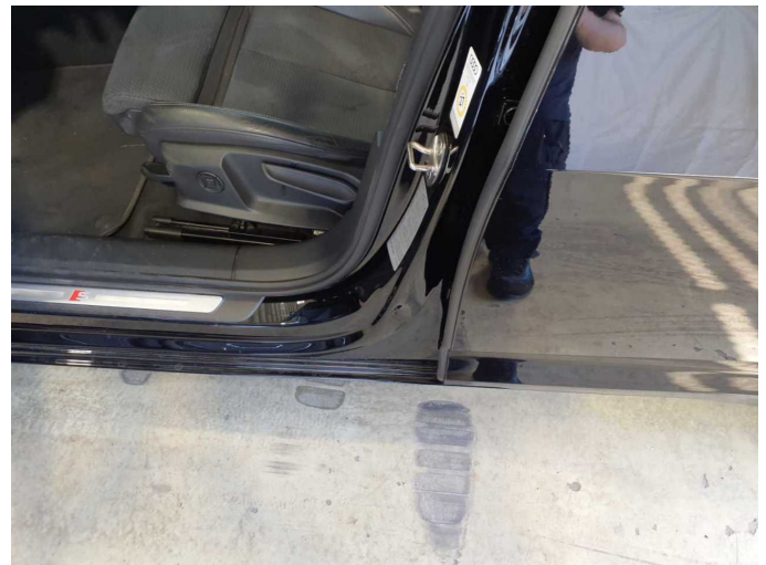
Damage 9: Body: B-pillar - left side - Deformed - Smart repair
