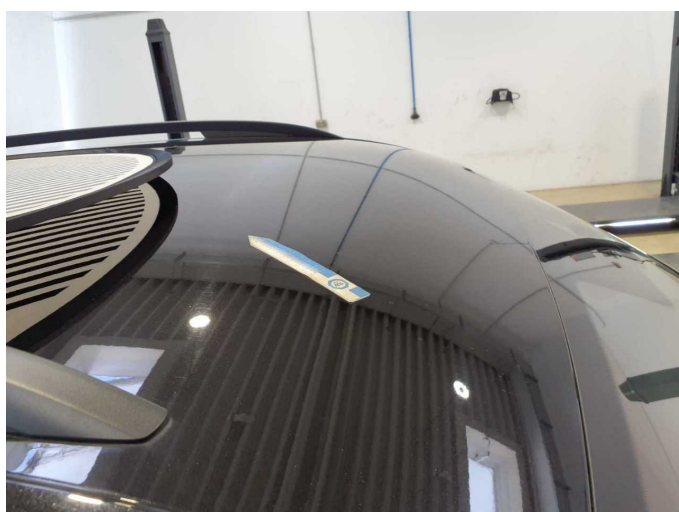
Damage 1: Roof: Roof - dent(s) - Smooth repair work
